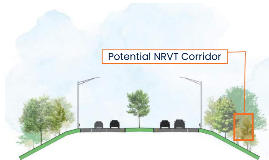
Route 7 Typical Section view looking North
